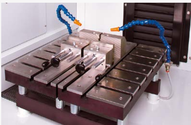
A spacious cutting chamber: W 408 x D 422 mm with openings on both right and left sides for the cutting of long samples.
