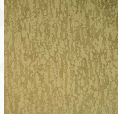
TA6V titanium etched by Kroll reagent
