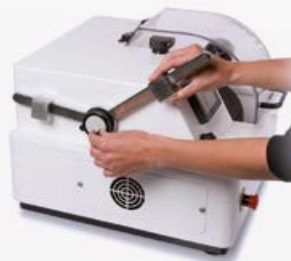
Manual micrometric adjustment of the Z axis.
