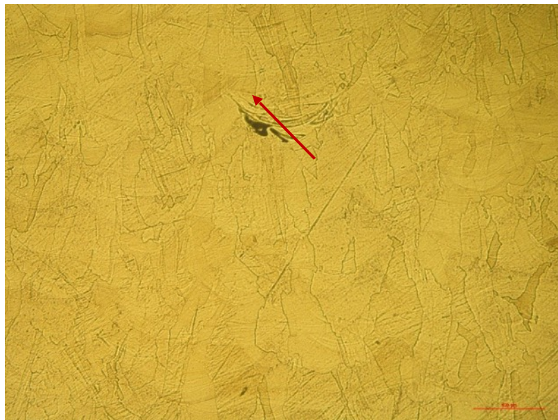
Microstructural defect (red arrow) from improper fusion of layers in additively manufactured steel 316L alloy.
