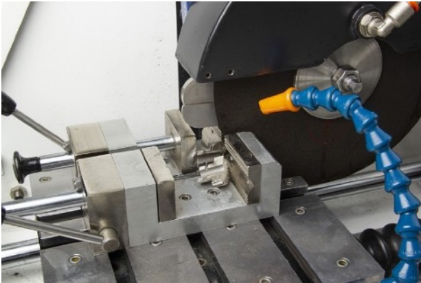
Additively manufactured piece (Steel 316L) cut using LAM PLAN Precision Red cutting wheel right through the feature of interest – hole perpendicular to the axis of the gear.
