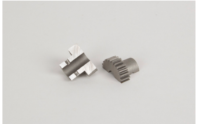
Additively manufactured piece (Steel 316L) cut using LAM PLAN Precision Red cutting wheel right through the feature of interest – hole perpendicular to the axis of the gear.
