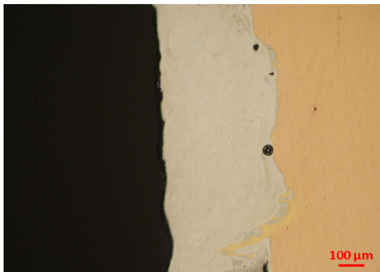
Microdefects revealed in copper-aluminum bonded layers after polishing on Touchlam 2T53 with Biodiamant Neodia 3P.
