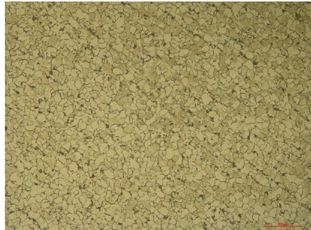
Microstructure of a rolled low carbon with regular but discontinuous bands of pearlite
