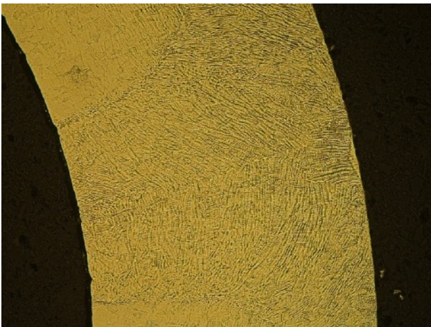
Austenitic grains in Stainless steel 316L from Additive Manufacturing (etched with Kalling's reagent)
