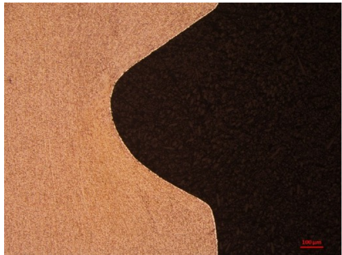
Microstructure of a surface treated titanium aircraft component (fastener) mounted in Epoxy 633 revealing the thin surface layer after etching with Kroll's Reagent.
