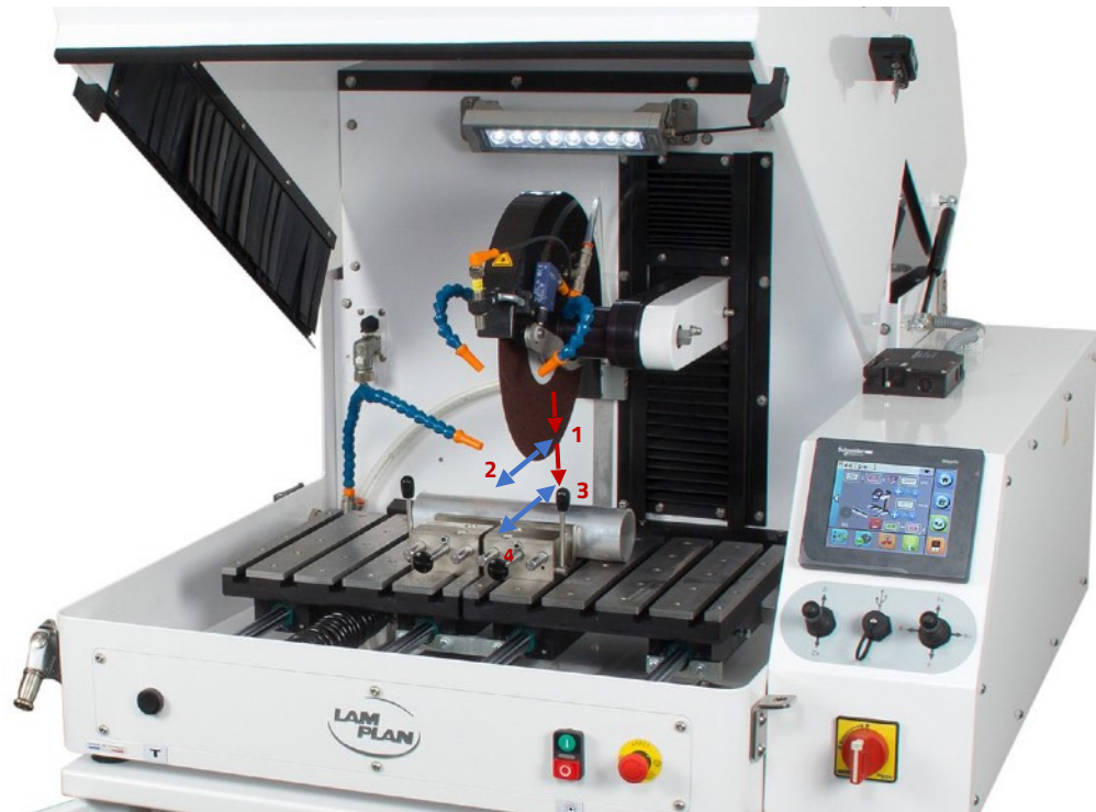
Y+Z cut performed on a cylindrical bar by moving the wheel and table alternatively as sequenced in the picture from 1 to 4.
